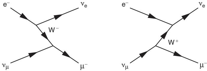
Fig. 5.3 The two lowest-order time-ordered diagrams contributing to  $e^- v_\mu \rightarrow v_e \mu^-$  scattering.
